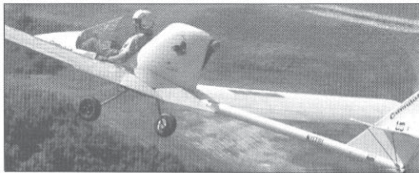
Although the roll response of the Cumulus was better than expected for a machine with more than 40 feet of wingspan, that response wasn't without noticeable adverse yaw. Lead with the rudder, though, and the Cumulus rewards you with a well-coordinated turn. The trick is in learning when and how much to lead.
