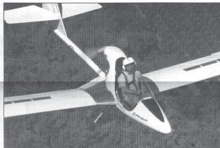
For a pilot-in-command seat sitting nearly in front of the cockpit, the Cumulus does an excellent job of protecting the pilot from windblast, thanks to the wrap-around windscreen that opens for cockpit access.
