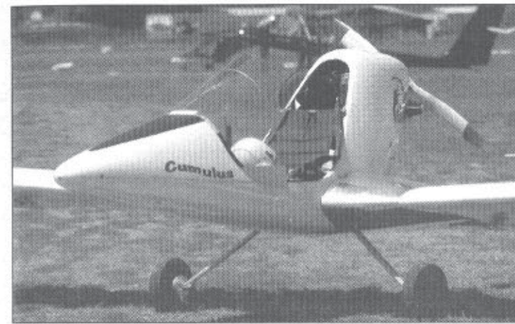
The simple, streamlined open cockpit gives the Cumulus pilot an unobstructed view of the world beyond his nose, while the sturdy conventional landing gear contributes the least possible drag to the ship's soaring mission while retaining a great deal of stability on the ground.
