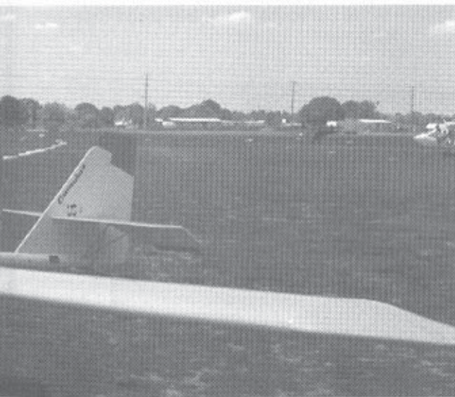
The key to the Cumulus' journeyman soaring qualities are in the wings: long and thin, with an effective airfoil profile. Spoilers help counter the qualities desirable for engine-off flight, expanding the variety of fields and approaches usable for landing.
