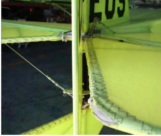
Rudder in Full right turn
